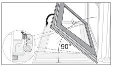
3. Fold up the clamping levers (A) on both door hinges back into their original positions.
